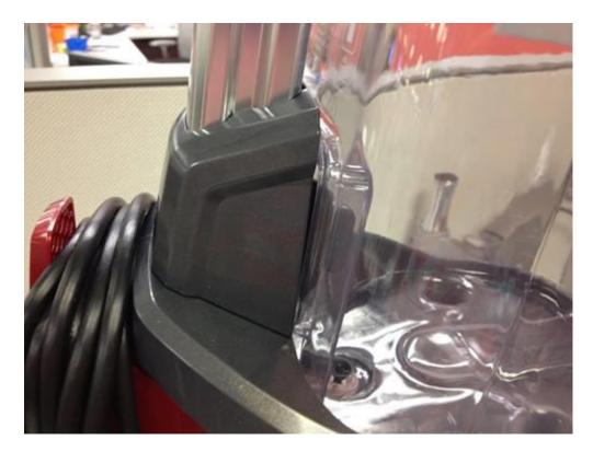
• Remove the hose and reconnect it. Be sure that the circular gasket on the hose is inserted into the circular opening on the foot and that the rectangular tab on the hose is inserted into the rectangular opening on the foot. The button should be facing outward.
