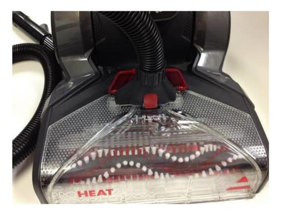
• If there is still no suction, remove the hose and check for cracks or other damage. Over a sink, run clean water through the entire hose to see if water will flow through it. If the water does not come through, a new hose is needs to be ordered.
