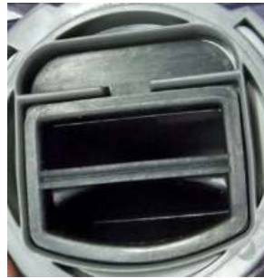
Gasket in tank (correct)
