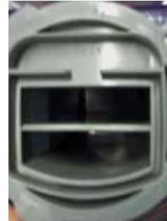
Gasket Missing (incorrect)
