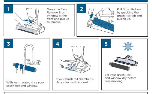
TIP: Running your machine with a wet Brush Roll will help it dry faster. The trigger should not be pressed.
