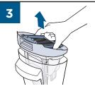
Grasp top of Dirty Water Tank in recessed areas on each side of the filter and pull upward to remove the top of the tank.
