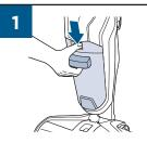
To release Dirty Water Tank, press down on recessed button on the top of the tank.
