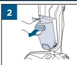
Grab the front handle while pressing down on the button and pulling the Dirty Water Tank away from the machine.
