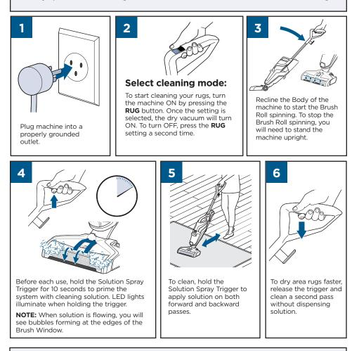
**NOTE:** The RUG button dispenses twice the solution of the HARD FLOOR button to help with area rug cleaning.
