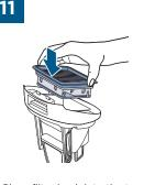
Place filter back into the top of the Dirty Water Tank.
