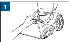
Lift the Accessory Hose Door on top of foot on the front of the machine. The door flips toward the machine to open.
