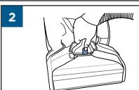
Insert the hose and snap into place. Be sure the coloured hose release clip is facing out, away from machine.
