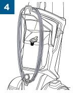
Wrap the cable around the Carry Handle and Cable Quick Release.
