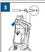
Using a Phillips-head screwdriver, secure the Carry Handle with the screw that's taped to the Upper Handle.
