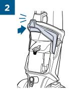
Next, align the Carry Handle with the slots on either side of the base (behind the Power Switch and Cleaning Mode Switch). The Carry Handle will "click" into place.
