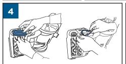
Remove the Brush Cover by lifting straight up. Remove the Cogged Large Pump Belt. The Brush Rolls can be replaced or cleaned at this time, if needed.
