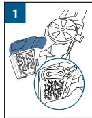
Remove Clean Water Tank and make sure the Dirty Water Tank is empty. Press the Recline Pedal and lay the machine on its side. Remove 3 screws on the belt/brush access plate using a Phillips-head screwdriver. Remove the plate to expose the belt.
