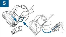
Now, if the Flat Pump Belt was broken, place a new Flat Pump Belt around the red area of the large pulley. Then use your thumb to stretch it toward the back of the machine and transfer it onto the metal axle.
