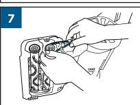
To replace the Cogged Large Pump Belt, make sure your deep cleaner is completely reclined. Begin by wrapping the Cogged Large Pump Belt around the small metal-toothed pulley. While wrapped around the pulley, stretch and wrap around the nearest brush gear.
