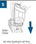
Upper Handle, align the Clean Water Tank with the grooves and slide the tank into place.
