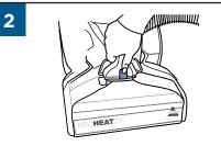
Insert the hose and snap into place. Be sure the colored hose release clip is facing out, away from machine.
