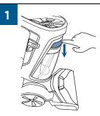
To release Dirty Water Tank, press down on the colored tank Handle.
