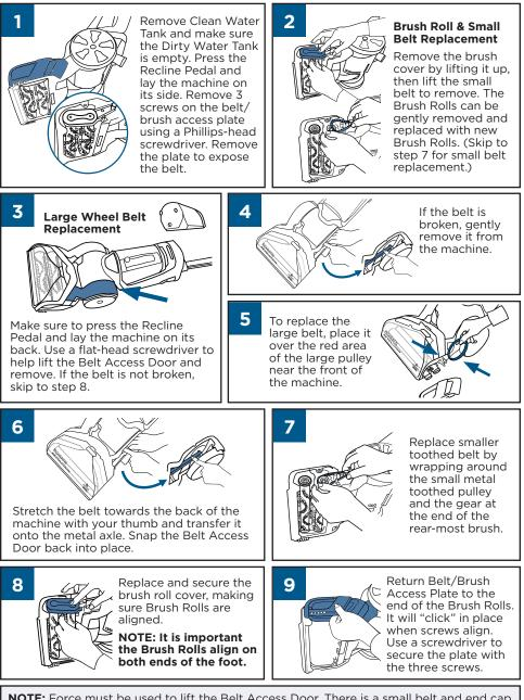
**NOTE:** Force must be used to lift the Belt Access Door. There is a small belt and end cap on the other end of the Brush Rolls. That belt needs to wrap around the tooth end of the Brush Rolls and the end cap needs to be secure before re-assembling the machine.
