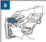
Return the Brush Cover. Make sure that the brushes are aligned and the cover is secure.
