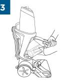
Pull Dirty Water Tank up and away to remove.
