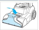
**9.** Reinstall nozzle, ensuring it aligns with slot on brush roll cover.
