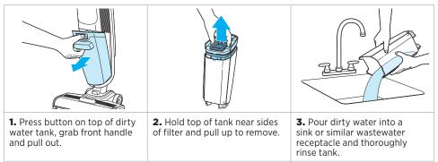
Note: Machine will automatically shut off the suction when the dirty tank is full.
