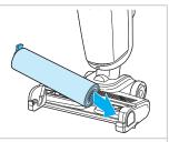
**3.** Reinstall brush roll. Place end of brush into right side of foot.
