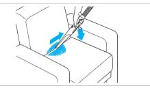
**2.** Release spray trigger and press tool firmly against surface and pull toward you to remove the stain. Repeat this step as needed.
